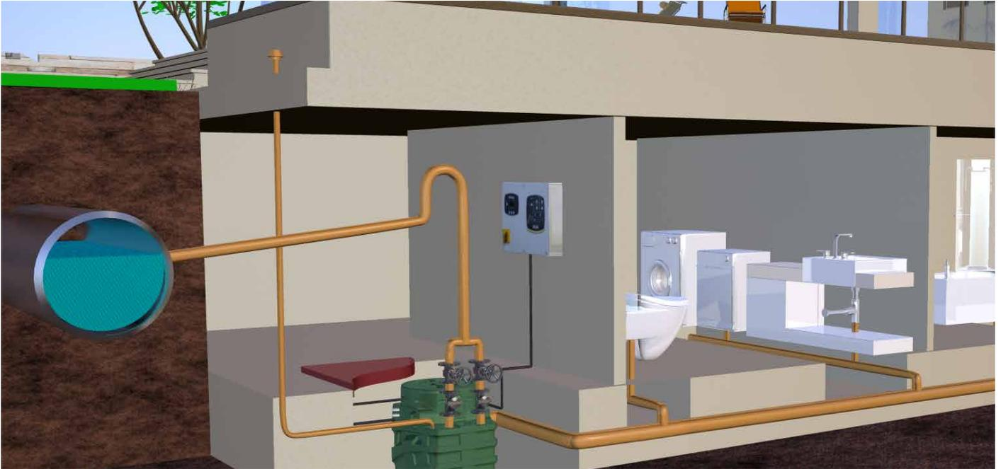
Ideal for piloting the pumping stations of filling / emptying the drainage of rainwater or waste water in general.
