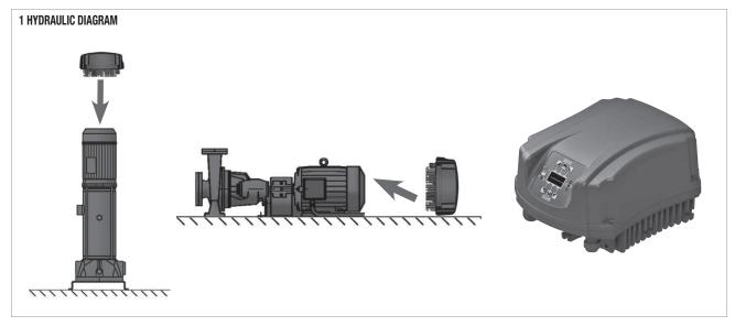
The MCE must be installed on the bottom of the motor. The inverter can operate both in the horizontal and the vertical position. 2 different kits for assembly on the motor are available:
